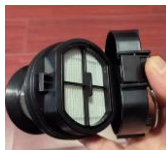
push button to take out the HEPA filter, pat or rinse in water, dry naturally
