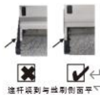
align the roll holder with the brush side
