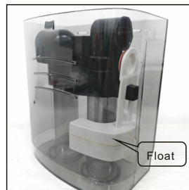
8. Please empty the dirty water before it exceeds the maximum water level line. If the water level exceeds the line and use continues, the float will activate and suction will stop. Note: When water seeps into the interior of the machine, please turn off the machine and clean the water inside the body, pipes, and water tank before using it again.
